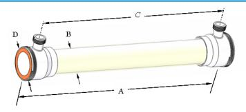
A B C D Permeate Process inches (mm) inches (mm) inches (mm) inches (mm) Connection 43 (1092) 5.0 (127) 38 5/8 (981) 6.0 (152) 11/2" NPSM 6" NPSM
