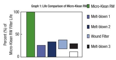
Consistent particle removal efficiency = improved R0 membrane protection The rigid Micro-Klean RW structure resists deformation, filter by-pass, compression and particle unloading. This allows Micro-Klean RW filters to achieve excellent filtration efficiency up to a differential pressure of 2.4 bar while other "flexible" competitive melt blown and string wound filters exhibit significant drops in removal efficiency at much lower differential pressures ( $\leq 0.68$  bar).
