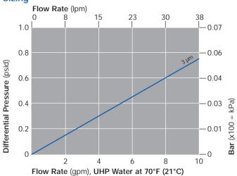
Flow rate is per 10" (25.4 cm) cartridge. For liquids other than water, multiply differential pressure by fluid viscosity (cP).
