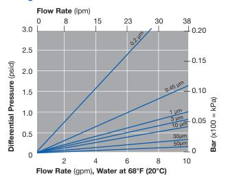
Flow rate is per 10" (25.4 cm) cartridge. For liquids other than water, multiply pressure drop by fluid viscosity (cP).
