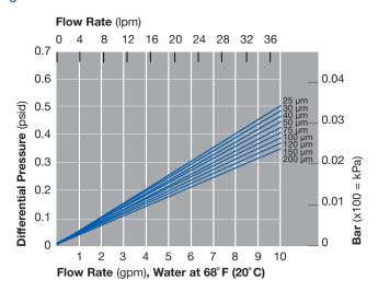
Flow rate is per 10" (25.4 cm) element. For liquids other than water, multiply differential pressure by fluid viscosity (cP).
