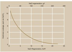
Capacity and Hardness Leakage graphs are shown assuming a service flow of 4 gpm/ft³ (32 l/h/l) and total dissolved solids of 400 ppm and 20 grains of total hardness. The hardness leakage will increase and the capacity will decrease while increasing total dissolved solids and total hardness.
