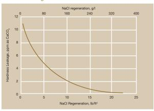
Capacity and Hardness Leakage graphs are shown assuming a service flow of 4 gpm/ft<sup>3</sup> (32 *VhV*I) and total dissolved solids of 400 ppm and 20 grains of total hardness. The hardness leakage will increase and the capacity will decrease while increasing total dissolved solids and total hardness.
